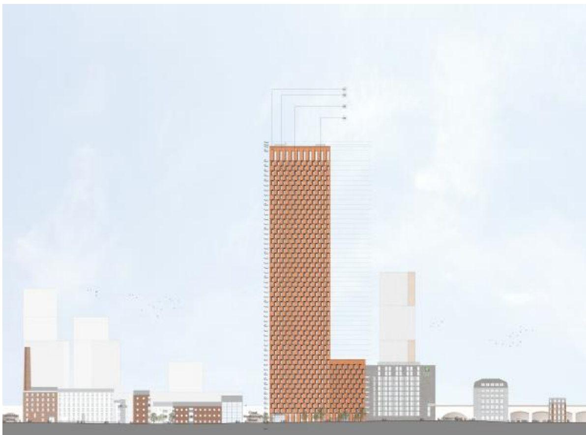
Hulme street elevation – showing deep regular window pattern and double height window to the crown of the building
